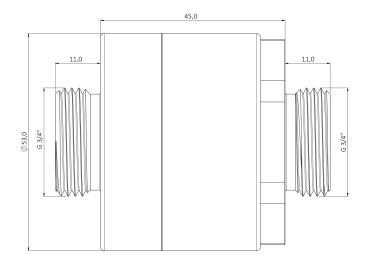
Note: dimensions as shown do not include sealing rings for installation
